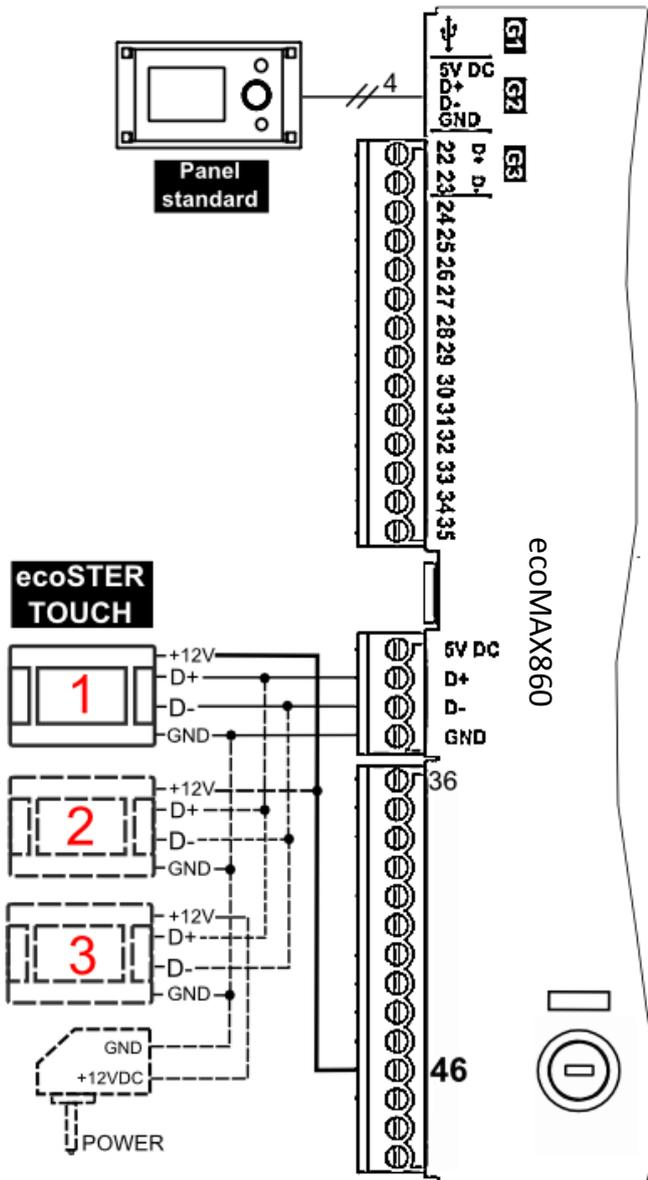
If the boiler controller is equipped with ecoTOUCH control panel (colored with a touch panel), only one ecoSTER TOUCH room panel can be supplied directly from the controller module (**socket G4**). Panels 2 and 3 have to be supplied by the additional power adapter **+12V, I ≥ 0.5A**.
