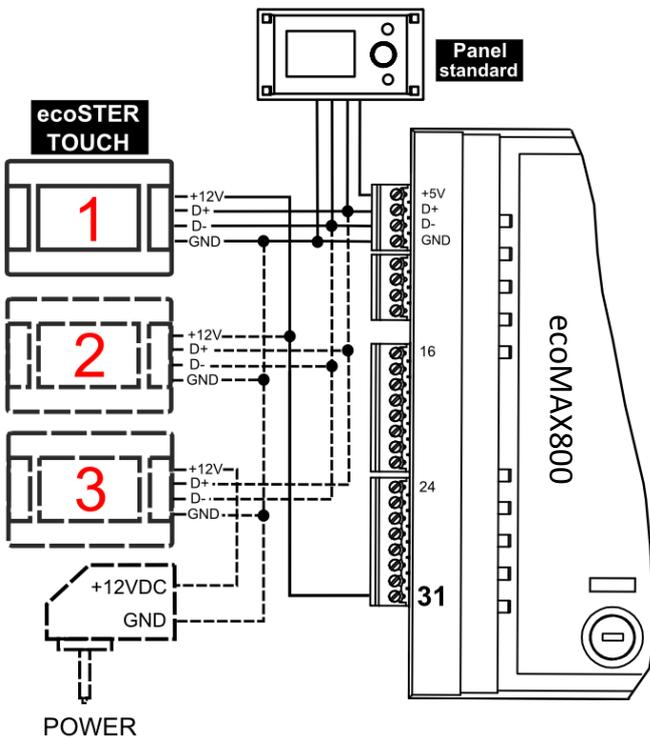
If the boiler controller is equipped with ecoTOUCH control panel (colored with a touch panel), only one ecoSTER TOUCH room panel can be supplied directly from the controller module (**terminal 31**). Panels 2 and 3 have to be supplied by the additional power adapter **+12V, I≥0.5A**.
